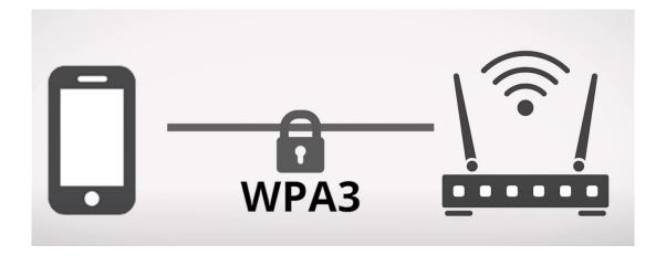
• WPA3 mandates the adoption of protected management frames, which guard against forging, and standardizes the 128 bit cryptographic suite and disallows obsolete security protocols.
