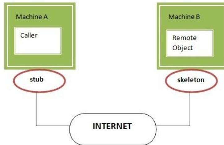
on the stub, the stub packages the method call and sends it to the server. The skeleton is an object that is created on the server side. It receives the method call from the stub and executes the method on the remote object. The skeleton then returns the result of the method call to the stub, which in turn returns it to the client.
