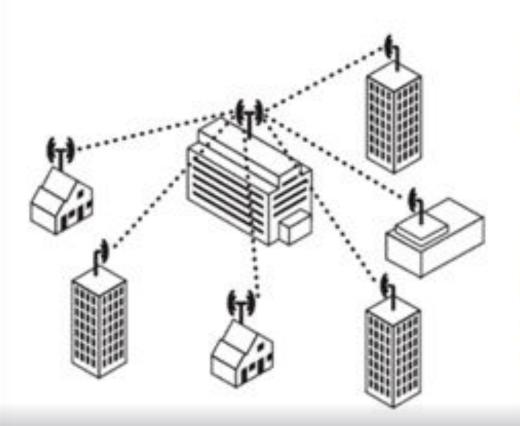
Instead of using point-to-point topology such as a mesh, LANs typically use a multipoint topology. The key to a multipoint topology can be summed up in a single word: sharing.
